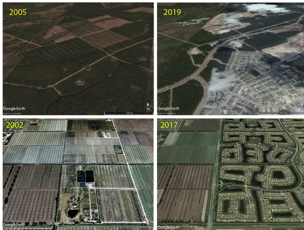
FIGURE 2 | Land use transitions to residential development highlight the use of wet detention ponds for stormwater management in the coastal zone. Upper panel: outside Charleston, South Carolina, 33^{\circ}3'33.01''\text{N} , 80^{\circ}8'48.85''\text{W} in the Sawmill Branch Creek watershed (HUC12: 030502010601); lower panel: outside Boca Raton, FL, 26^{\circ}30'35.22''\text{N} , 80^{\circ}11'29.72''\text{W} , in the Hillsborough Canal watershed (HUC12: 030902061101). Stormwater ponds in the two developed panels to the right side are visible in the form of dark areas surrounded by homes/buildings. In the upper-right panel, two large ponds are visible near the center, while many ponds (round or elongated) are visible in the lower-right panel. Upper-right panel, through partial cloud cover, also shows expansion of new developments with clear cutting and re-grading of the pre-existing managed-forested landscapes, and a borrow pit is found in the top-left corner. The lower-left panel also shows (at bottom-center) prior agricultural use of ponds.
